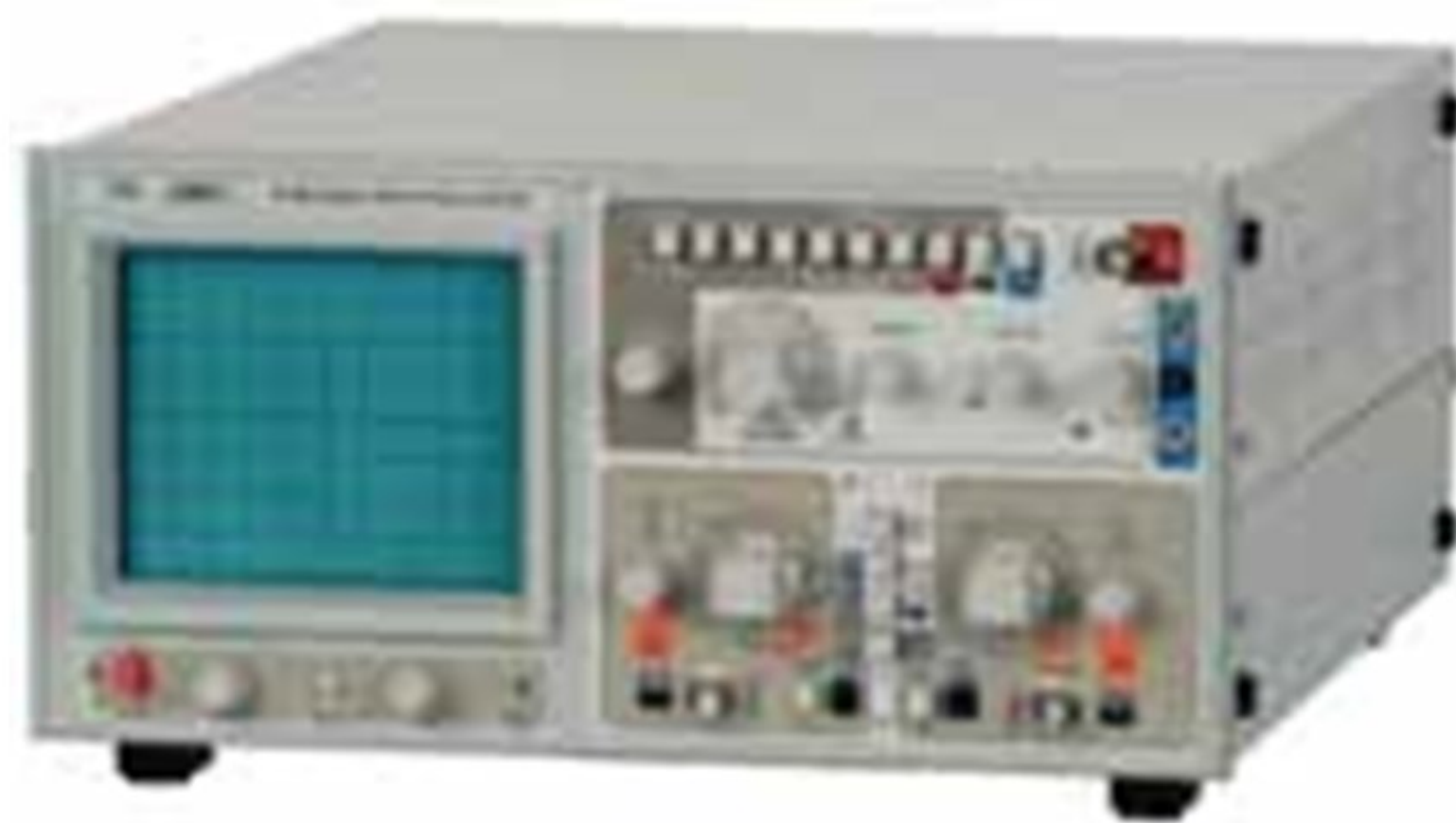
Figure 2.35 A two-channel laboratory CRO (photo courtesy of Philip Harris)
