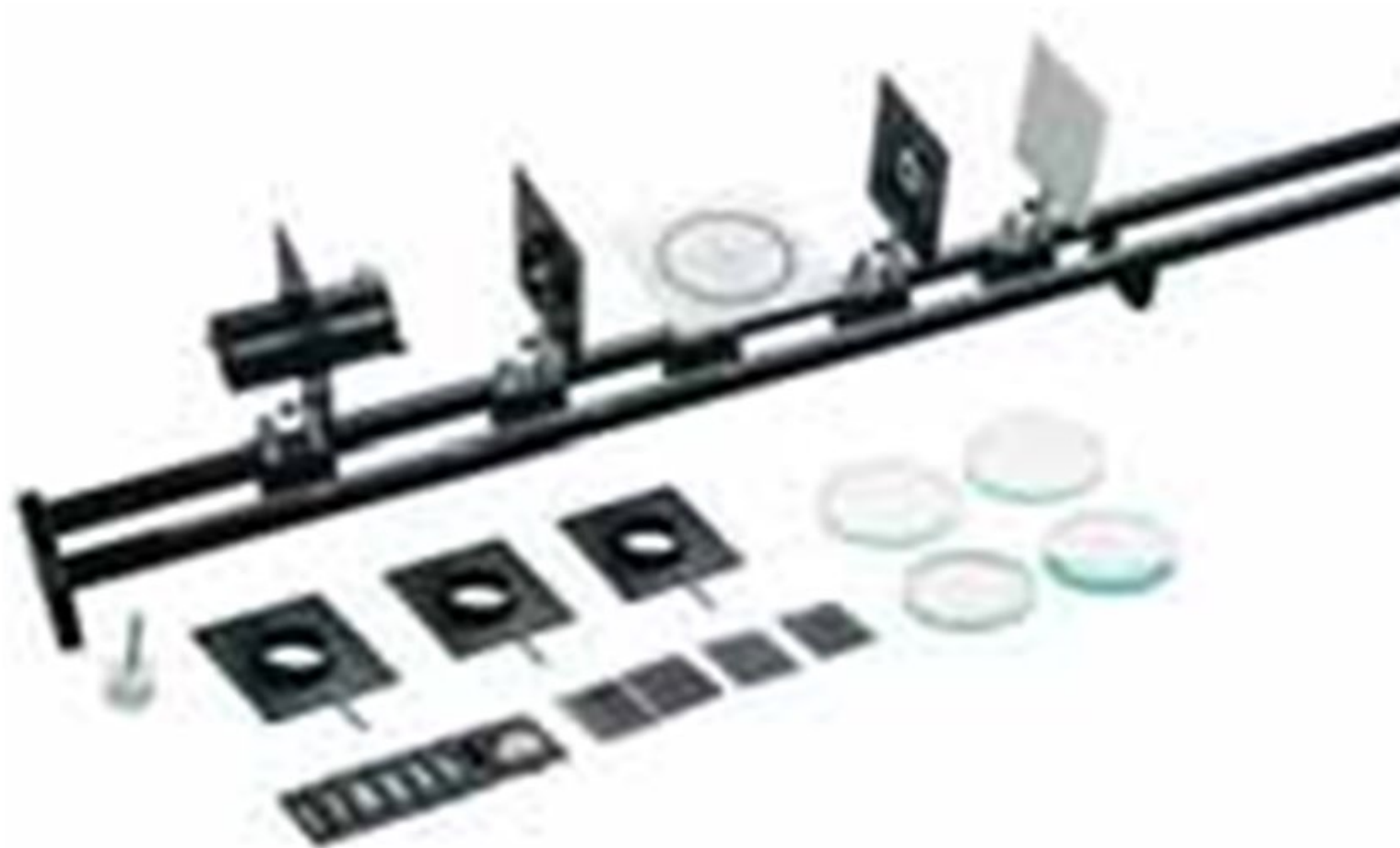
Figure 3.11 An optical bench with lenses (photo courtesy of Philip Harris)
