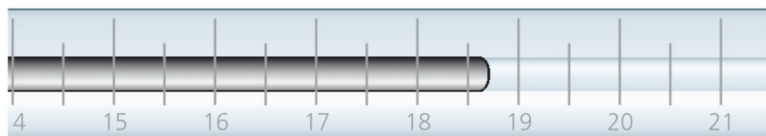
Figure 5.1 A magnified thermometer scale showing a temperature of 18.7°C: the last digit is uncertain
